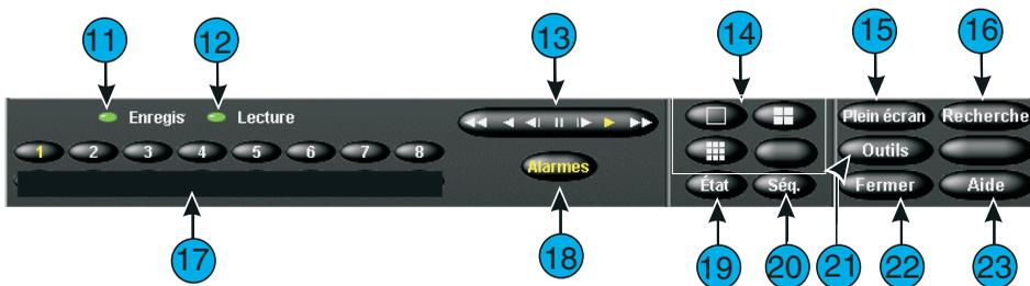
Figure 10 — Playback Controls and Indicators
