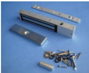
**637.008.401** 261-000 Non-Monitored Single Magnet 12 or 24V DC (Nominal 480mA@12v DC.) for internal Door Up to 250KG Holding force
